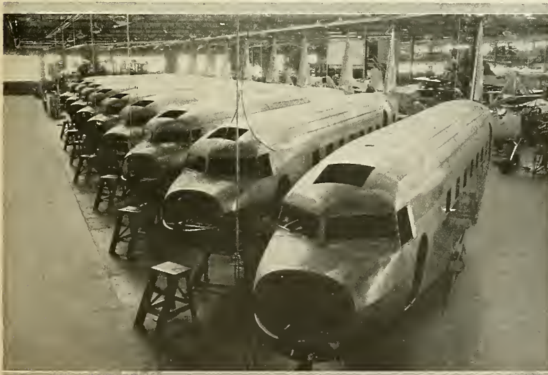
Douglas transports on the fuselage assembly line in the Santa Monica factory
